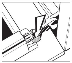
■ Push down the locking clamps on each door hinge.
